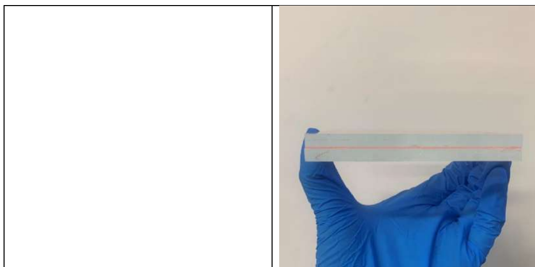
Figure 1 Fabricated LSC samples showing flexible substrate laminated between two sheets of low-iron glass
